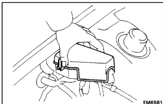
**11. REMOVE IGNITER COVER, AND DISCONNECT CONNECTORS**
