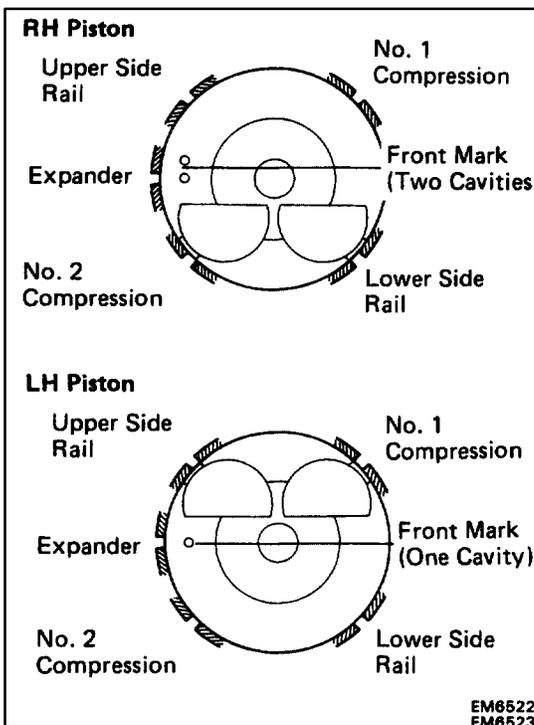
(c) Position the piston rings so that the ring ends are as shown.
