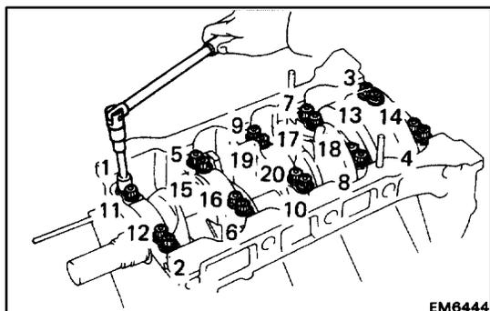
(b) Uniformly loosen and remove the twenty main bearing cap nuts in several passes in the sequence shown.
