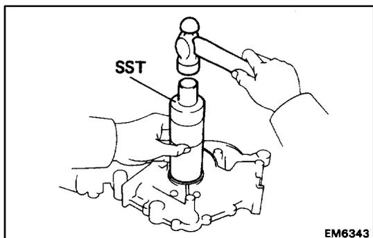
(b) Using SST and a hammer, tap in a new oil seal until its surface is flush with the oil pump case edge.
