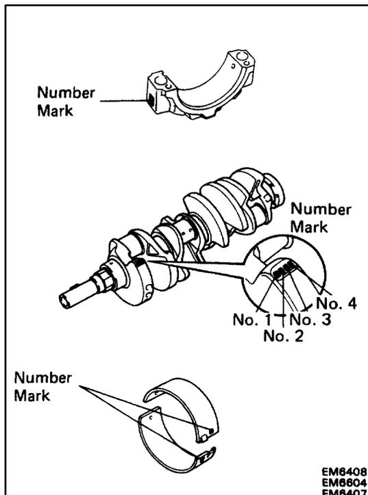
HINT: If using a standard bearing, replace with one having the same number. If the number of the bearing cannot be determined, select the correct bearing by adding together the numbers imprinted on the connecting rod cap and crankshaft, then selecting the bearing with the same number as the total. There are six sizes of standard bearings, marked “2”, “3”, “4”, “5”, “6” and “7” accordingly.
