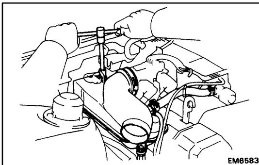
**20. INSTALL INTAKE AIR CONNECTOR PIPE**
