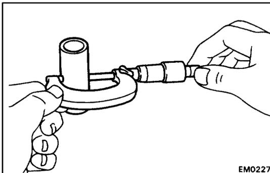
(b) Using a micrometer, measure the piston pin diameter.
