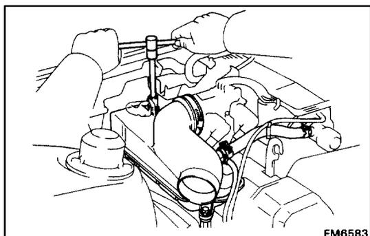
**13. REMOVE INTAKE AIR CONNECTOR PIPE**
