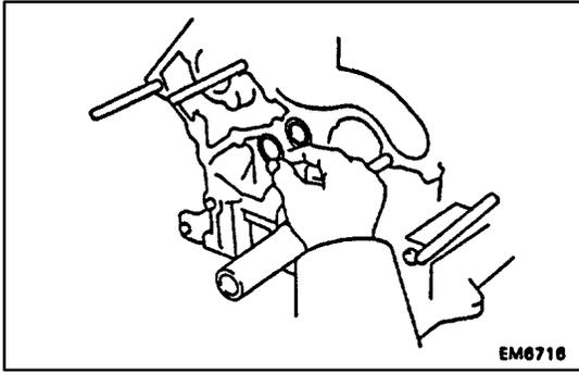
(c) Place a new O-ring in position on the cylinder block.
