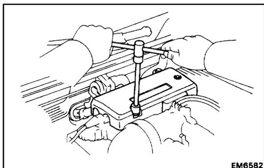
**12. REMOVE THROTTLE BODY COVER, AND DISCONNECT CABLES**
