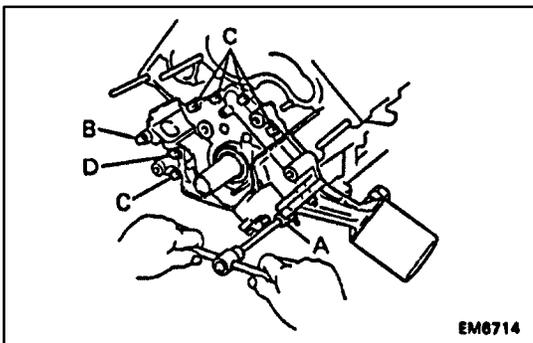
(e) Install the oil pump with the eight bolts.
