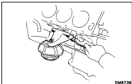
5. **REMOVE ENGINE MOUNTING BRACKETS**
