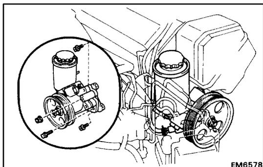
**14. REMOVE PS PUMP WITHOUT DISCONNECTING HOSES**
