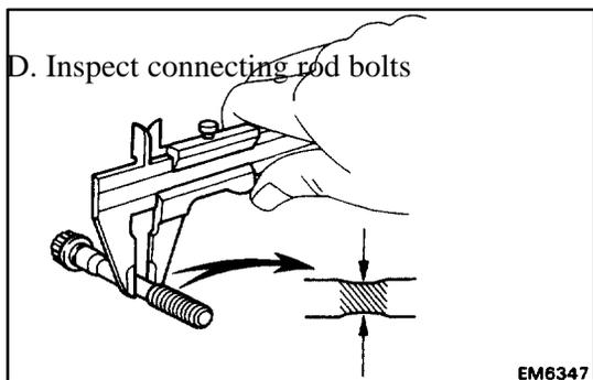
Using vernier calipers, measure the tension portion diameter of the bolt.
