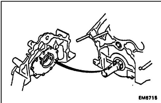
(d) Engage the spline teeth of the oil pump drive gear with the large teeth of the crankshaft, and slide on the oil pump.
